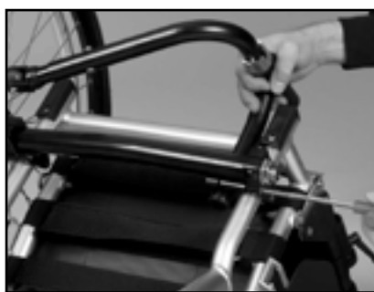
Fig. 41 Juster anti-tip sikringen
