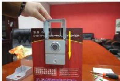
8. Slip the rain proof cover from up to down
