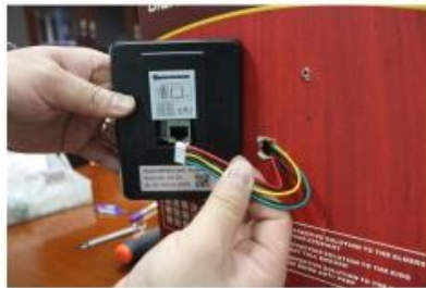
4. Connect to the power wire
