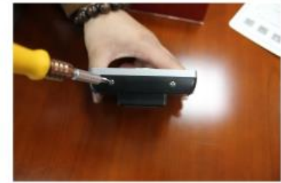
3. Unbolt the wifi doorphone outside panel
