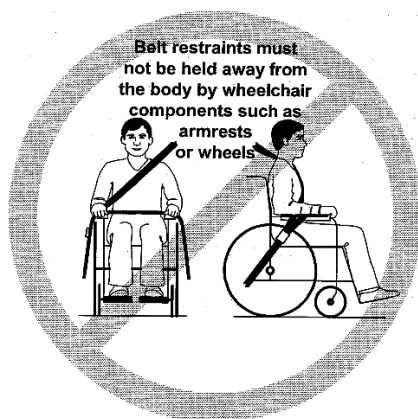
Figure 6 — Illustration of improper belt-restraint fit
