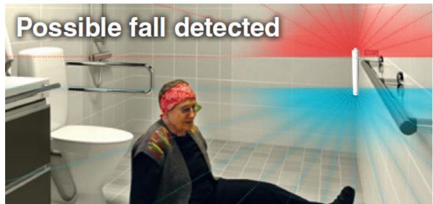
Figure 3.5 Only the Bottom PIR Sensor now detects the Person, triggering an Alarm
