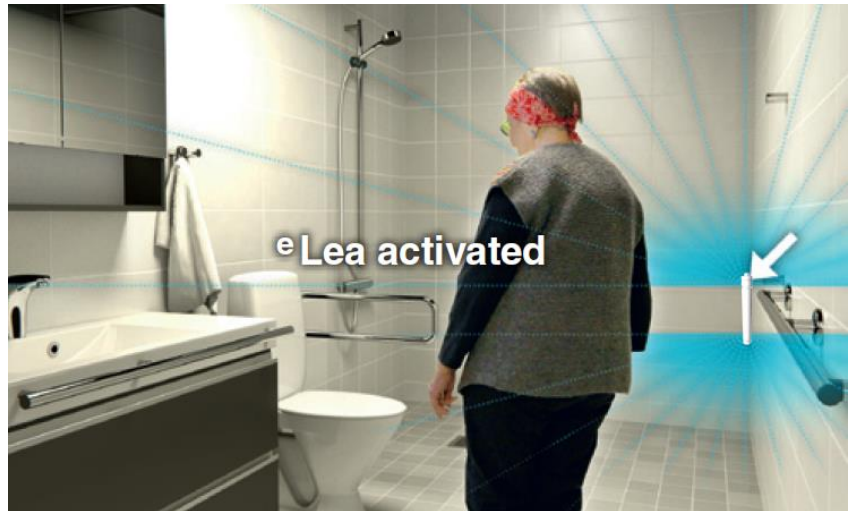
Figure 3.4 Both Bottom and Top PIR Sensor detects the Presence of a Person
