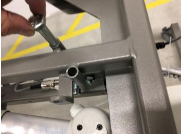
29. Slide the back section onto the joint flaps and secure the hinge bolts. Make sure that the plastic bearings in the outer link plates are not lost.
