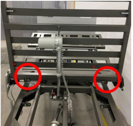
30. Fold up the back section, remove the motor bolts from the motor fork head from the transport bracket, pull out the lifting tube as far as it will go, insert it into the motor abutment on the back section, replace the motor bolts and secure them. Fold down the back section again.
