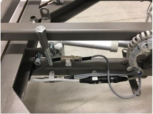
19. Connect the cable couplings of the two lifting units.
