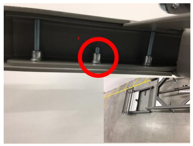
22. The lower part of the bed frame can now be inserted in the transport trolley with the footrest facing up and outside. Unscrew the adjustable feet beforehand and reinstall them in the respective holder.
