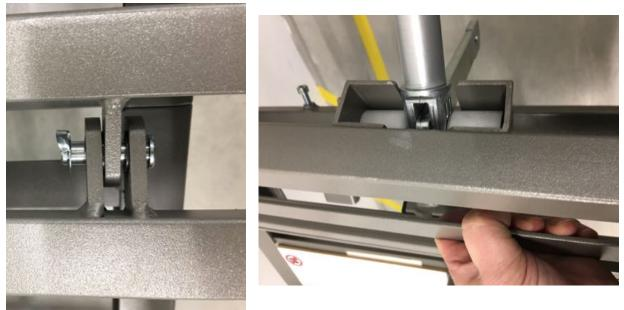
5. Remove the splint pin from the axle bolt on the swivel frame, unscrew the knurled nut and pull out the screw.
