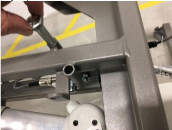
3. Remove the two motor bolts on the rotation motor. Then remove the rotation motor from its abutments and pass it to the other side under the central beam of the rotation frame.
