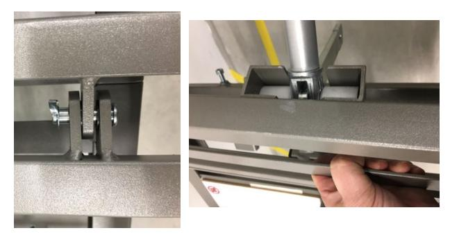
10. Slightly press the swivel frame at the head end against the direction of rotation so that the rotating stop pin can be removed. Now pull out the motor bolt from the rotary motor on the axis of rotation and insert the motor clevis into the holder underneath and replace the motor bolt.
