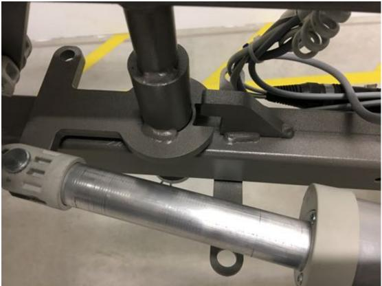
28. Insert the rotary stop pin on the opposite side to the rotary motor into the mounting sleeve. Press the rotation frame slightly against the rotating direction until the rotating stop pin falls completely into the sleeve.
