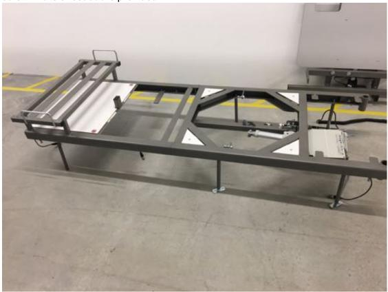
5. Fold up the back section by hand, unhook the upper engine bolt, fold down the back motor, slide in the lifting tube and insert the clevis head into the provided holder and secure it with the engine bolt.
