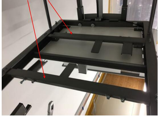
27. Remove the bolt of the rotation motor. Then remove the rotation motor clevis from the transport holder and attach it to the rotation lever on the rotation axis. Reinsert and secure the motor bolts.
