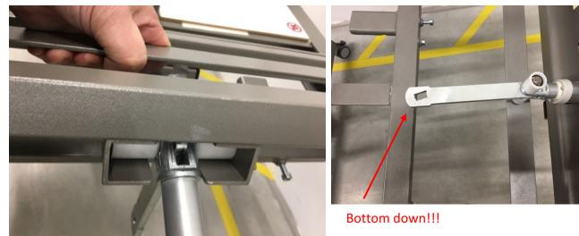
32. Insert the lower leg section into the upper leg section and insert and secure the hinge pins. Then insert the leg section motor coupling rod into the housing on the lower leg section, insert and secure the hinge bolts.
