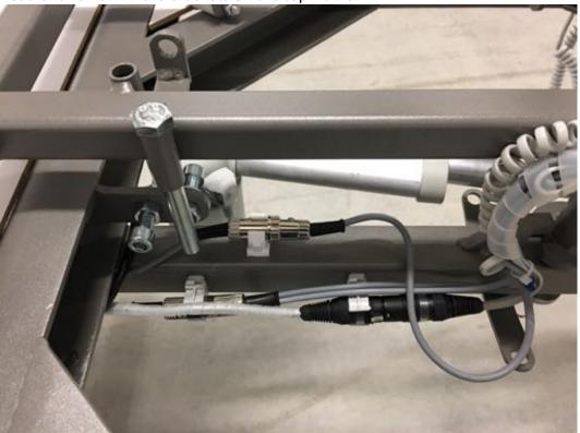
18. Disconnect the cable coupling from the lifting motor at the head and foot ends and disconnect the cable coupling at the middle frame separation point.
