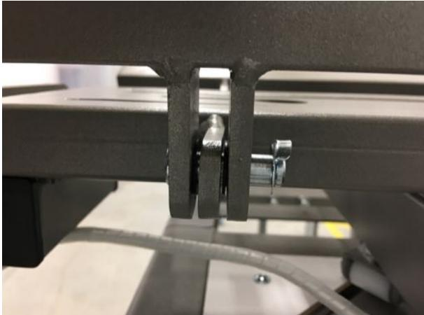
7. Remove the hinge pin from the motor coupling rod, on the lower leg section.
