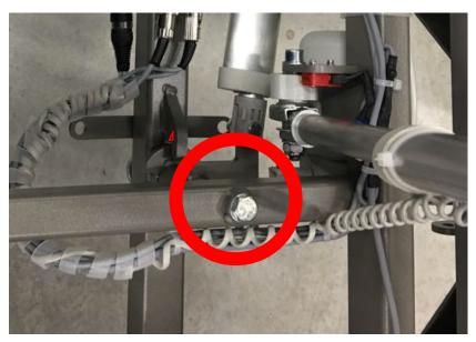
6. Remove the swivel frame from the axle tube.
