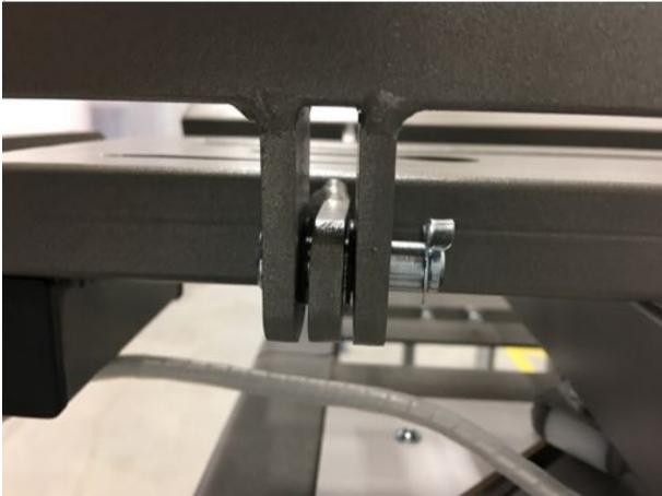
4. Remove the hinge pins of the lower leg section and the leg section motor coupling strut and. Then remove the lower leg section and replace the joint pins.
