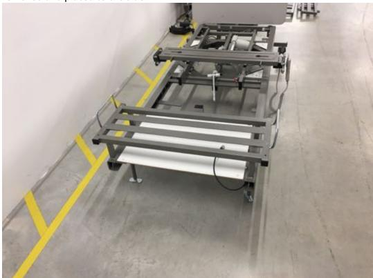
20. Head and foot ends can now be connected by means of the transport devices and their locking screws are screwed in.
