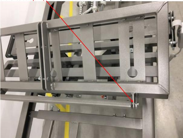
Remove the hinge pins from the upper leg section. Then remove the upper leg section from the lifting motor. Reinsert the hinge pins and secure them for storage. Place the lifting motor leg section on the frame and leave the coupling rod and guide rollers (secured by toothed pulleys) on the frame.
