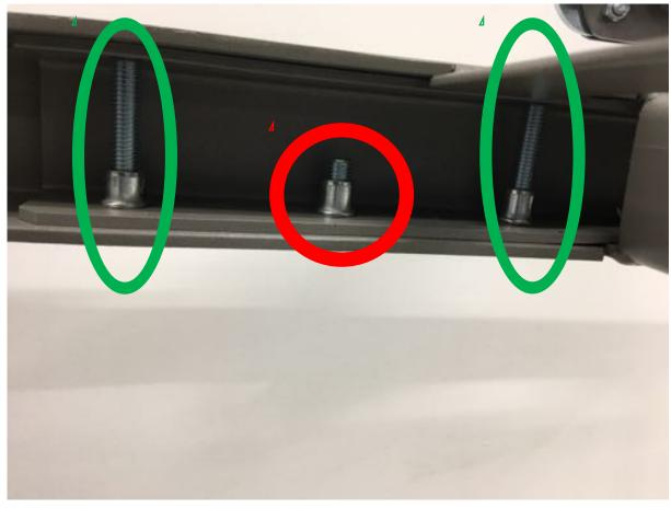
24. Tighten the four screws M10 at the head and foot ends of the bed frame and the two M8 locking screws.
