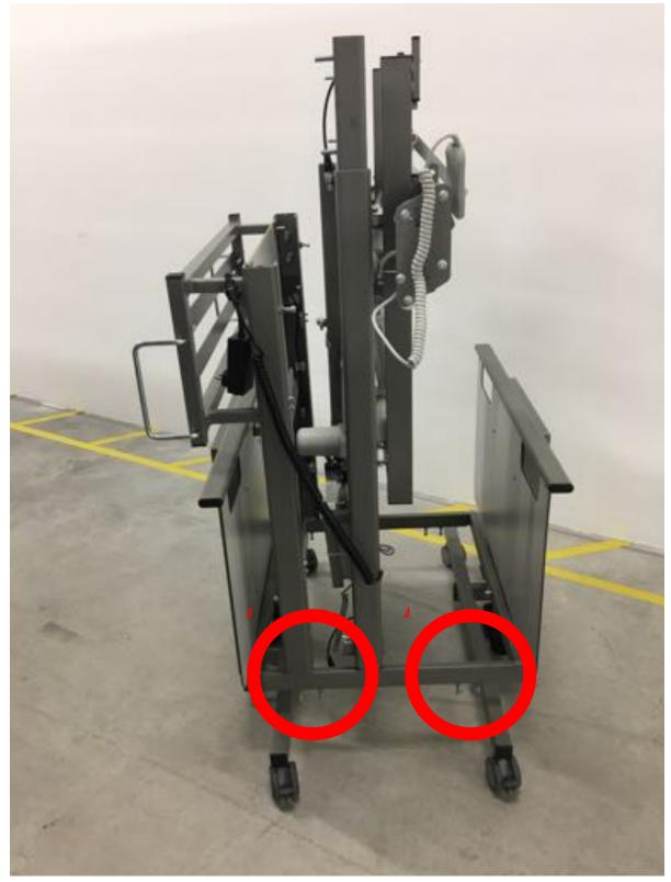
15. Attach the lifting units to the head and foot of the bed frame.
