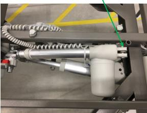
6. Fold down the back section, remove the two hinge pins, remove the back section and replace and secure the motor bolts in the hinge plates.
