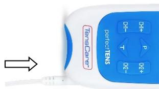
**Attaching the electrode pads to the lead wire.**
