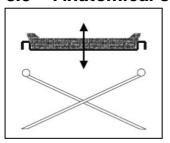
If you have opted for an anatomical padded seat, place it on the tubular cross-hinge so that the seat's supports engage equally with the cross-hinge. In the wooden base you will find slots that are placed in the hinge's cross-pieces. To fold up the wheelchair, remove the seat by pulling it upwards.
