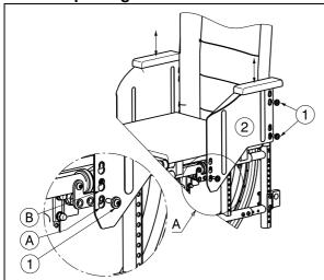
The armpads of the wheelchair can be adjusted in 2 different positions.
