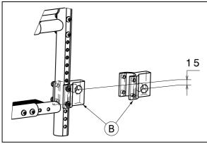
It is also possible to rotate the rear axle block B (2 positions: steps from 15 mm).
