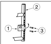
The driving wheels are mounted in an axle adapter  $\odot$  at the bottom of the back frame  $\circ$ .
