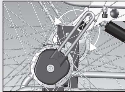
Brake of manual wheelchair in neutral position
