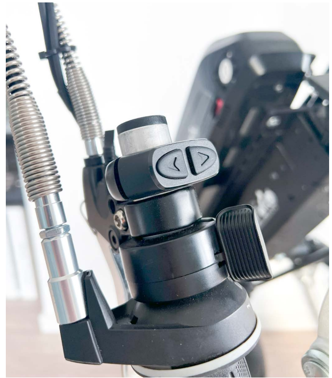
Fig. 26: Thumb throttle and display control unit
