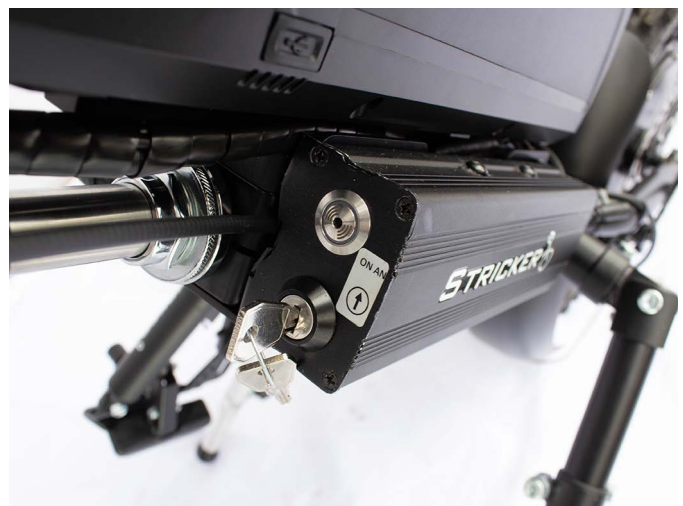
Fig. 12: Key switch on battery and control
