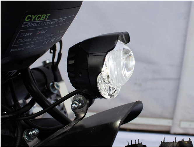
Fig. 31: Adjustment of the inclination of the lamp with integrated horn
