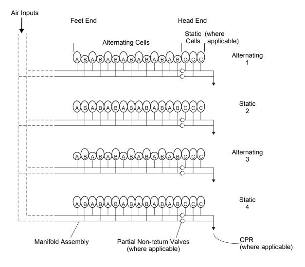
Figure 4 - Typical Mattress Pneumatic Diagram and Cell Inflation Cycle
