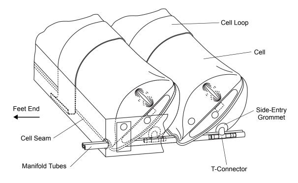
Figure 25 - Cell Orientation
