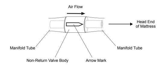
Figure 23 - Orientation of the Non-Return Valve Assembly
