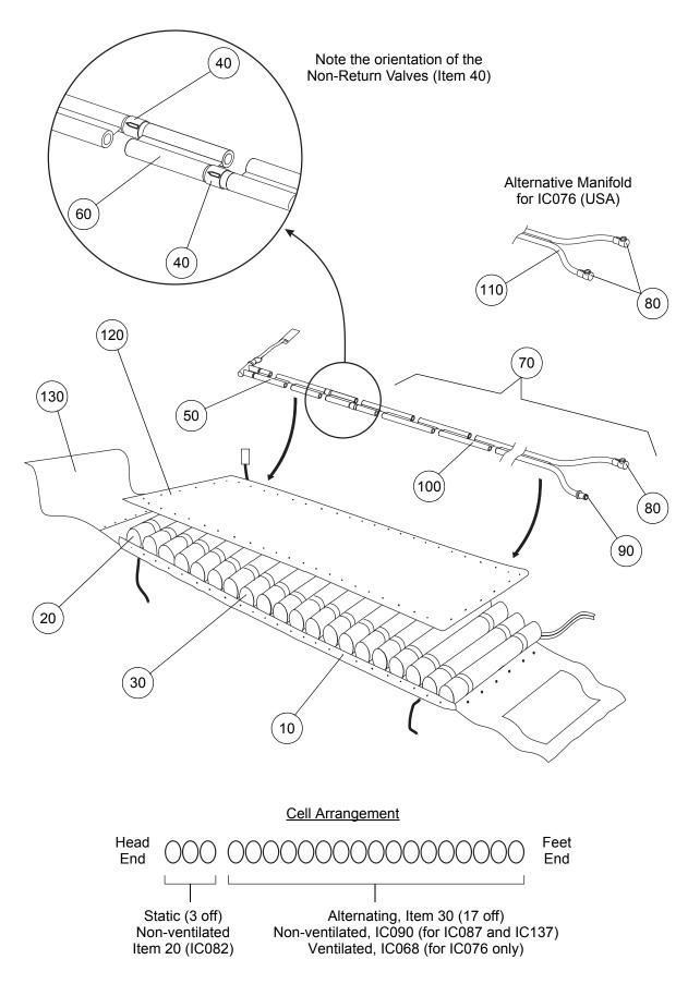
Figure 12 - AlphaXcell Mattress Overlay (OL)
