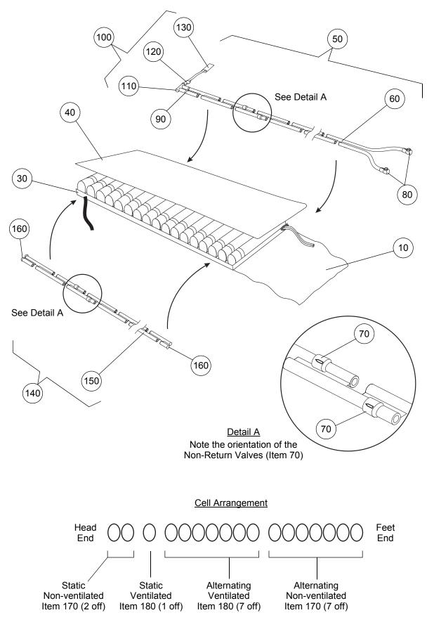
Figure 7 - Alpha Active Mattress Overlay (OL)
