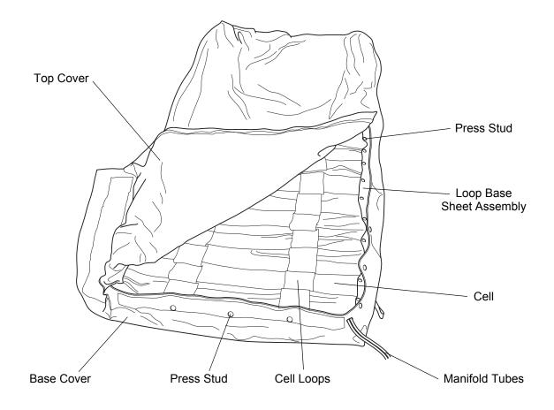
Figure 22 - Removing the Top Cover (typical view)
