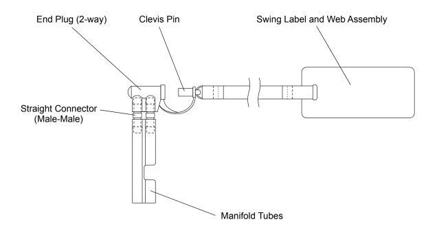
Figure 26 - CPR/Rapid Deflate End Plug Assembly
