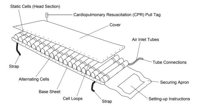
Figure 1 - Typical Mattress Overlay (OL) System
