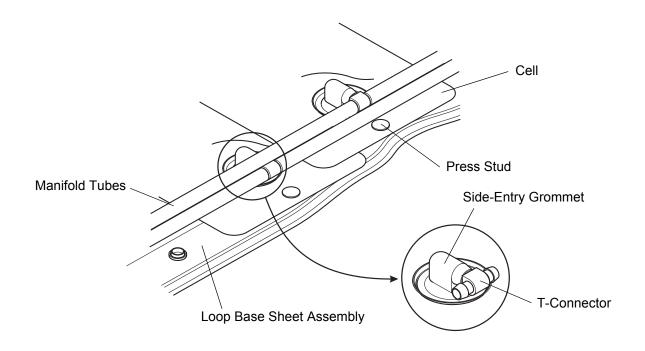
Figure 24 - Manifold - Cell Connections
