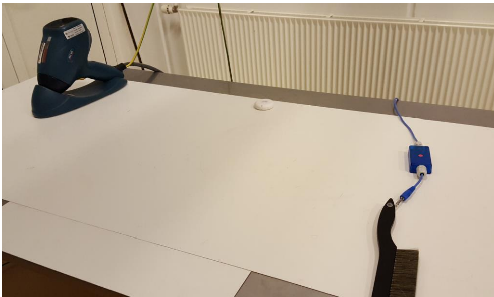
Photo 6. Electrostatic discharge test setup.
