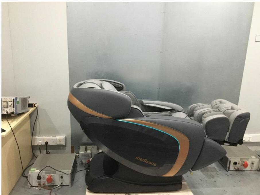
Radiation Emission Test View (Below 1GHz)
