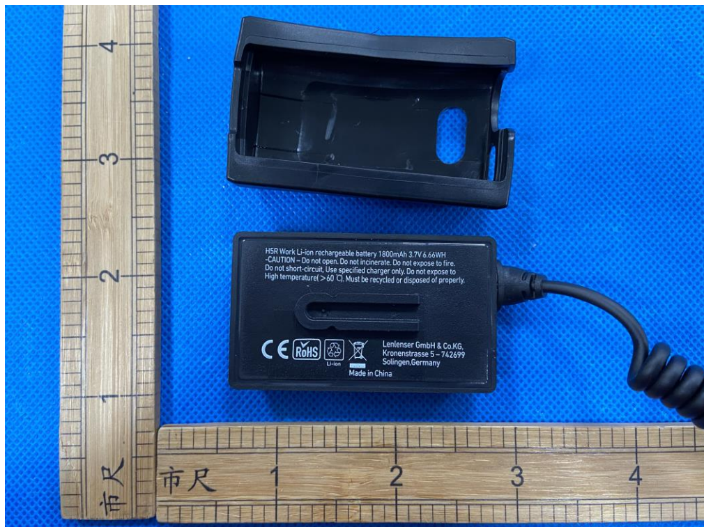
Figure 6. Overall view of Battery
