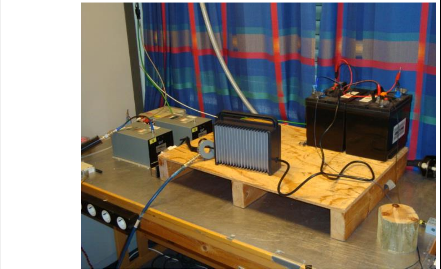
Notes: Test set-up for Conducted RF Disturbance
