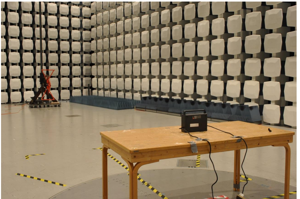
Notes: Test set-up for Radiated Emissions
