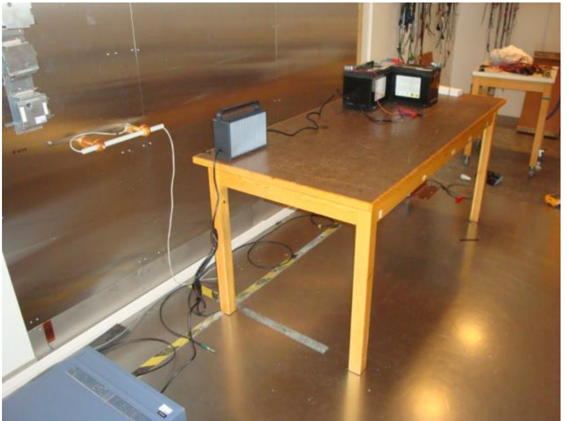
Notes: Test set-up for Conducted Emissions
