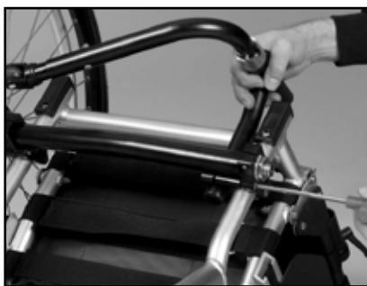
Fig. 33 Juster anti-tip sikringen
