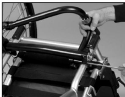
Fig. 41 Juster anti-tip sikringen
