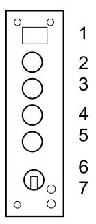
Is the platform not on the level on which you want to move onto the platform, you can call the platform by using the wall controls:
