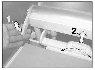
After pulling the desk out of the table body and setting it to the horizontal position it can be also adjusted in height. After taking up the lever of the lock in arrow 1 direction the desk is released and it can be set to required position pulling it up.
