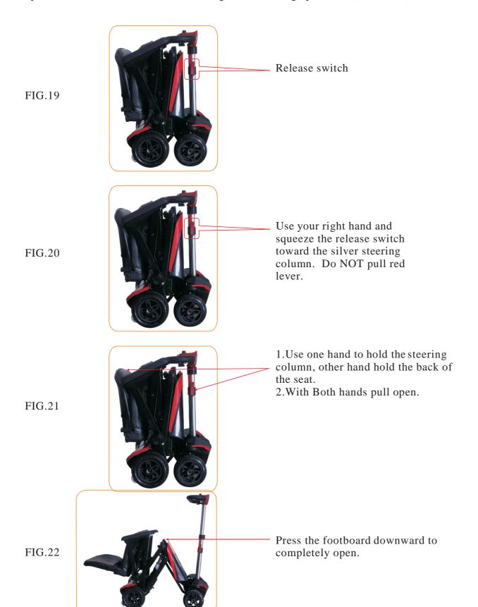
Note: If the scooter was closed by the remote control, than it must be opened by the remote control. The manual release will not work.
