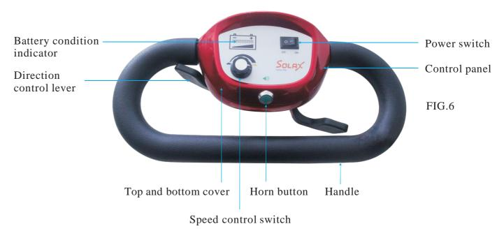
Notice: Be sure to always protect the Transformer control panel from humidity and water. If the control panel has been affected by moisture, be sure to dry before operation.
