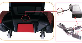
Then open the rear charging socket and insert the plug
