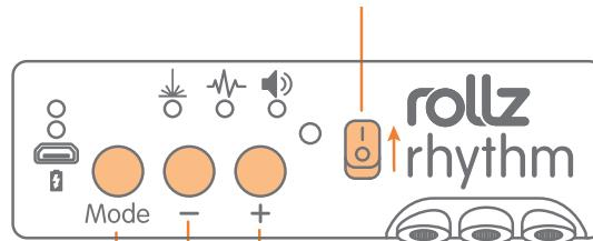
Use “-” and “+” buttons to increase or decrease the walking frequency in steps/min. For a slower walking speed, press “-”. For a faster walking speed, press “+”.
