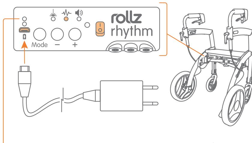
The module will display a red light while charging. When fully charged, this light will turn green. Charge the module only with an adapter of 5V and 1A.
