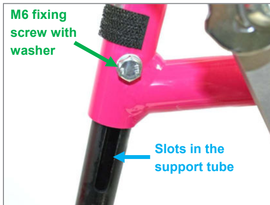
Figure 97: M6 fixing screw with washer and slot in footrest support tube for adjusting the lower leg length
