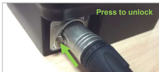
Figure 157: Unlocking the charger plug
