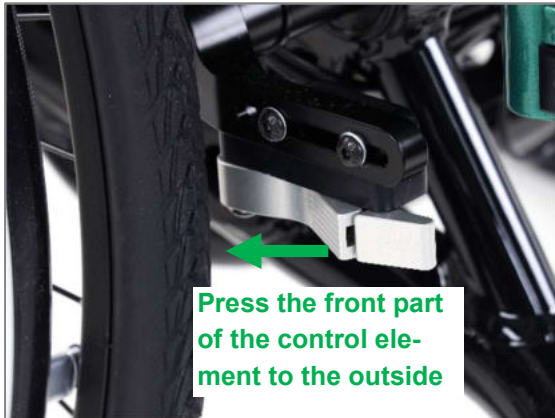
Figure 132: Integral brake open, closing is carried out by pressing the control element outwards
