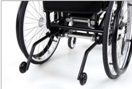
Figure 114: Operating position of anti-tipping support (view from the rear)
