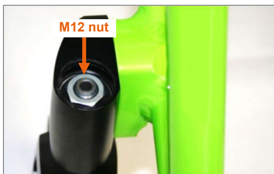
Figure 75: Aluminium cap removed and M12 nut visible
