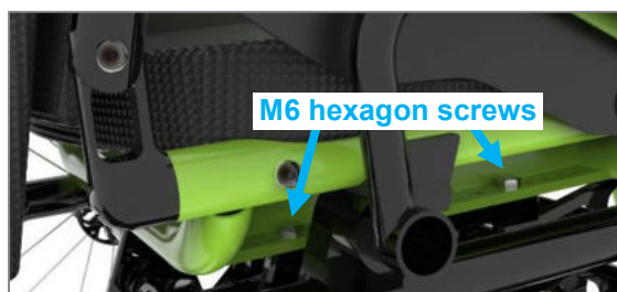
Figure 4: Seat unit with hexagon screws
