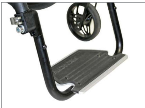
Figure 86: Footrest, fold up to the rear, in standard position
