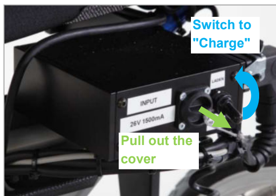
Figure 158: Preparation for charging at the rear of the wheelchair
