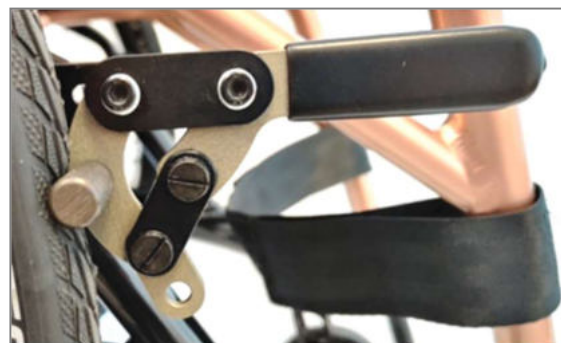
Figure 118: Knee lever brake system with standard brake lever
