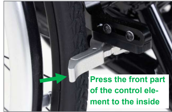
Figure 134: Integral brake closed, the brake is opened by pressing the control element towards the middle of the wheelchair
