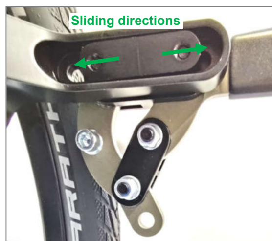
Figure 121: Sliding directions (LIFT activ; view from the inside of the wheelchair)
