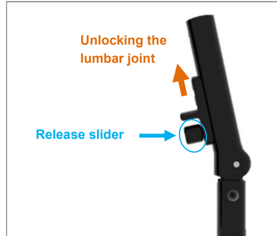
Figure 17: Lumbar joint with release slider
