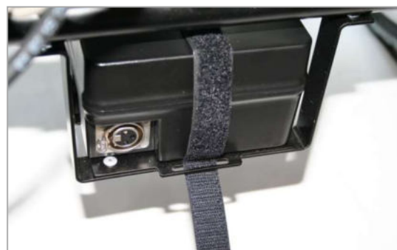
Figure 160: Open the Velcro band, Step 1
