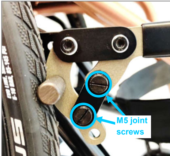
Figure 126: M5 joint screws for setting the actuating force of the brake lever (installed at the front)
