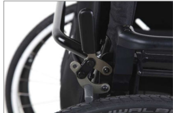
Figure 128: Knee lever brake installed at the rear (view from the side)
