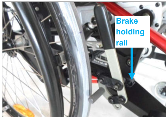
Figure 123: Knee lever brake (low assembly position), long brake lever; LIFT solid
