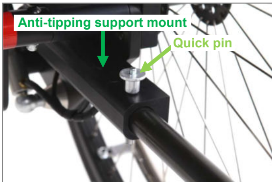
Figure 115: Anti-tipping support with quick pin (view from the rear)
