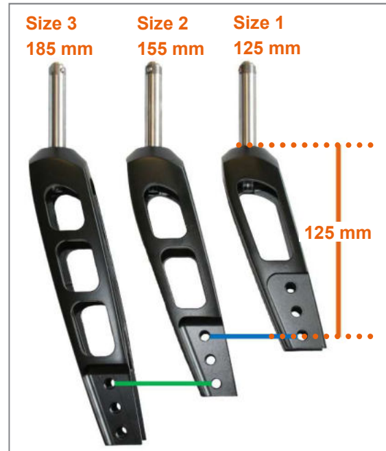
Figure 2: Caster fork sizes with marking of the same seat height settings with different caster fork sizes
