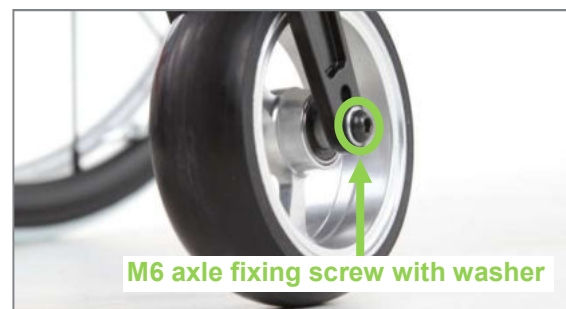
Figure 68: M6 axle fixing screw of caster wheel axle (view from outer side of product)
