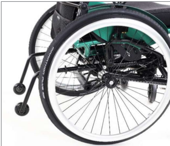
Figure 110: Operating position of anti-tipping support (view from the side)
