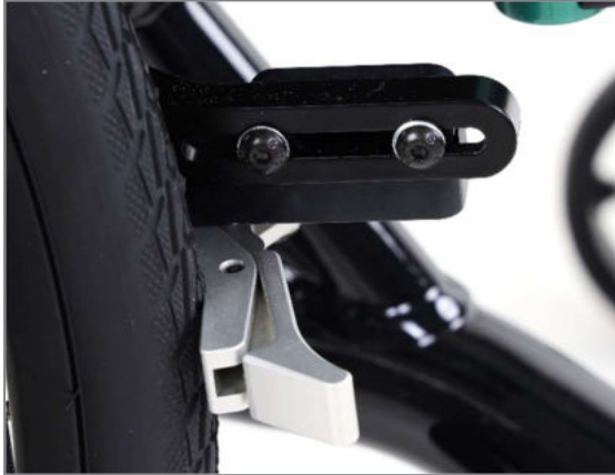
Figure 135: Brake element resting on the tyre
