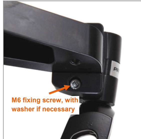
Figure 81: M6 fixing screw on frame inner side, washer fitted with G-shape frames but not V-shape frames
