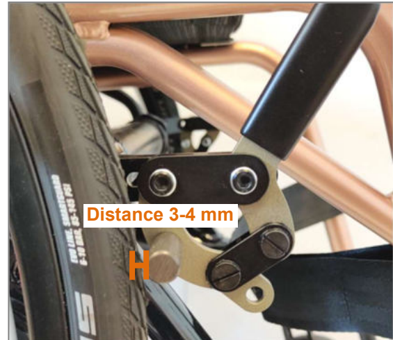
Figure 125: Distance between the brake pin and tyre of approx. 3 to max. 4 mm with the brake opened (installed at the front)
