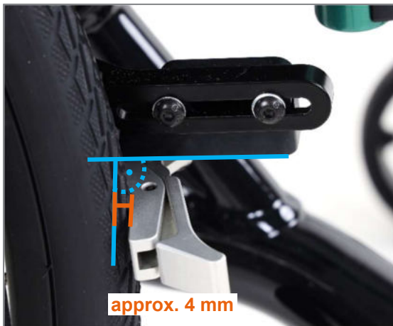
Figure 136: Brake element after correct positioning of the integral brake
