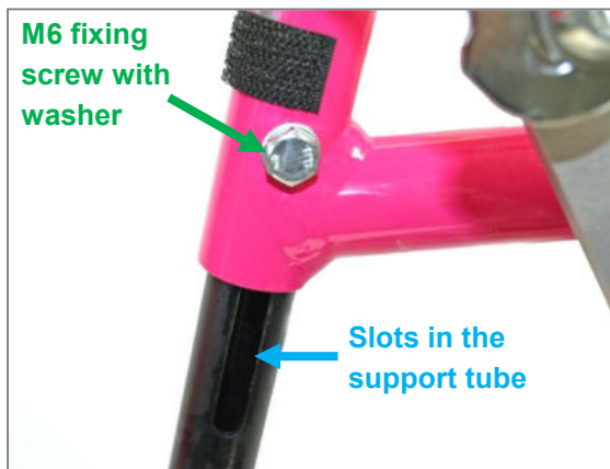
Figure 100: M6 fixing screw with washer and slot in footrest support tube for adjusting the lower leg length
