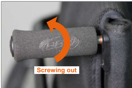
Figure 140: Screw the push handle horizontally out of the back tube
