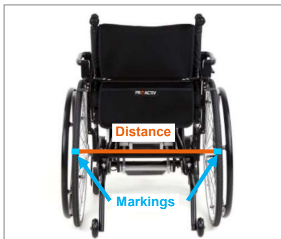
Figure 56: Distance between the markers on the tyres (at axle height), (view from the rear; LIFT solid)
