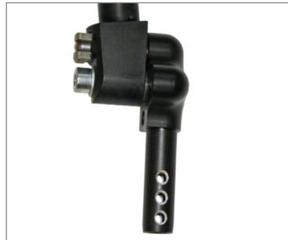
Figure 91: Inlet with 3 holes (view without footrest support tube)
