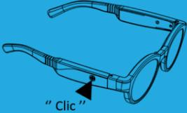
Press the ON/OFF button for 3 seconds. The bluetooth is activated when the LED on the right temple flashes blue. The LED turns fixed blue when the Lexilens® frame is connected to your smartphone application.
